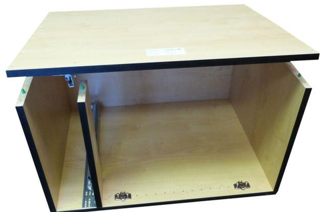
**6. Clamp the box together**, using bar-type clamps, top-spanner type clamps or a case clamp. A suggested clamping technique is shown below:
