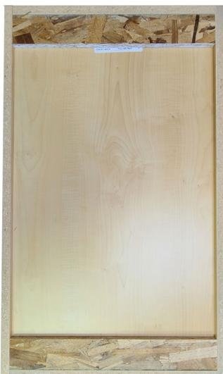
**7. Release clamping pressure** after the glue sets (normally, 20 minutes is ample for DD060 doweling glue or a thinned PVA-type glue but assembly in areas of high humidity may require longer clamp time).
