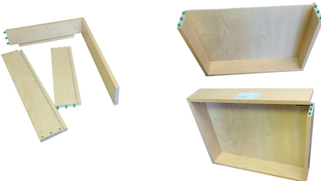
12. When assembly of the drawer box has been completed, if using Tandem slides, turn the drawer box over on a protected surface and install the two locking devices at the front (no notches) of the box. Screws are included for installing the devices. Locking devices will screw into the inside front edges of the box if using solid wood or plywood boxes and pilot drilling is recommended. (Shown in the Tandem adjustment section, below)
