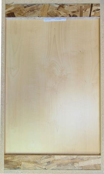
**7. Attach the OSB nailer strips** to the back of the cabinet. Base and wall cabinets have two nailers, one at the top and one at the bottom, recessed so they are flush with the cabinet sides. Tall cabinets will have three nailers, with the center one usually being set just below a fixed shelf.
