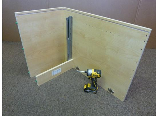
**4.** Insert the top and bottom panels, along with any drawer rails or fixed shelves, into the corresponding pre-bored end panel, using the dowels to align and loosely hold the parts. Then install **Confirmat Screws** snug, but not yet tight, through the counter-bored holes in the end panel.
