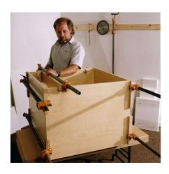
Always check the box for square prior to setting the clamps and do not apply excessive pressure with any type of clamp. The corner blocks direct the clamping force without bowing the panels. A coating of wax in the inside corner will prevent glue from attaching to the blocks. Sets of 4 each of 12", 21" and 24" blocks will cover most cabinets and should last for years.
