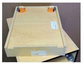
If splitting is encountered, you can try removing the hardware and prying the split sections apart very slightly - a toothpick used as a wedge can help separate the material – gently does it! Then force glue into the crack, clamp the material back together, and wipe off excess glue.
