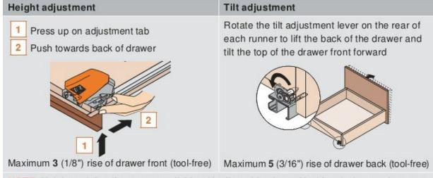
NOTE: Height and tilt adjustments available with all combinations of locking devices and runners
